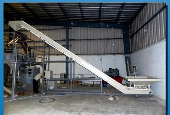
Z Belt Conveyor
